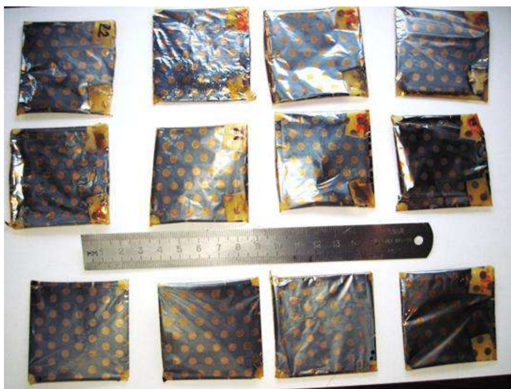
Fig. 1. General view of thin-film ITO/CdS/CdTe/Cu/Au PVC samples.
