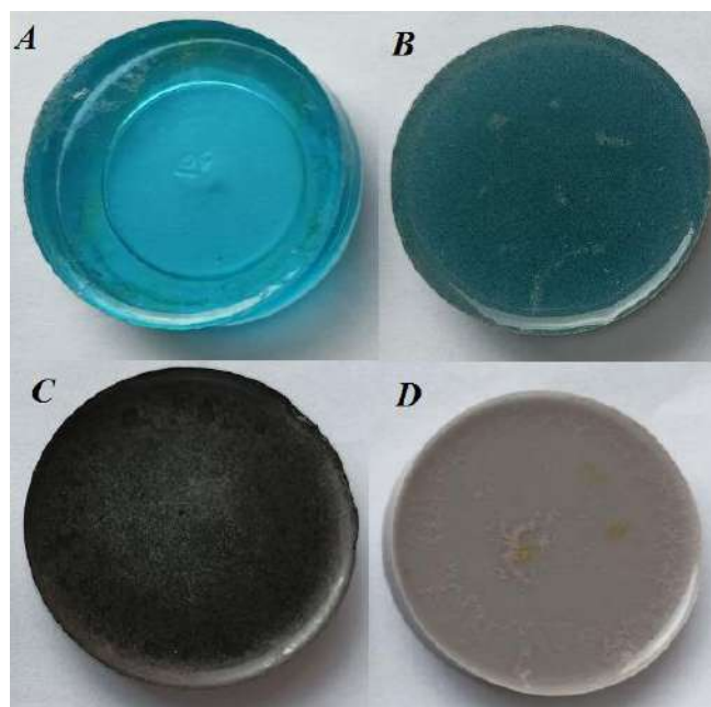
Fig. 1. Photo of polymer ceramic-inorganic composites: A – pure epoxy resin; B - epoxy resin with 20 % wt. SiC; C - epoxy resin with 10 % wt. graphite +10 % wt. Cr 2 O 3 ; D - epoxy resin with 20 % wt. potassium titanates.
