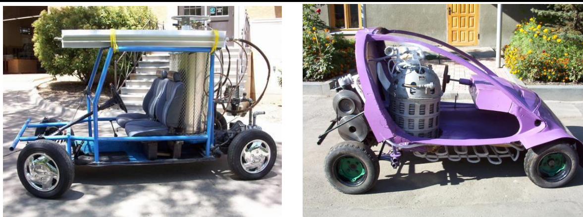
Fig. 3. Liquid nitrogen powered prototype vehicles, built by a) UNT (left), b) Kharkov research team (right)
